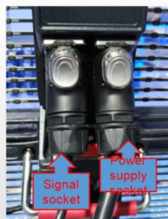
Power box navigation, signal navigation docking
