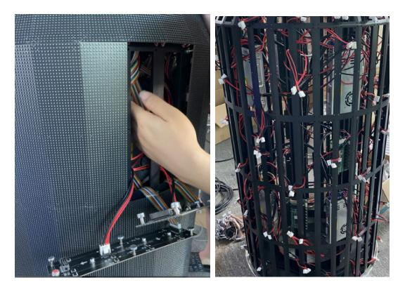
All parts including the power supplies, receiving cards and modules can be front maintened.
